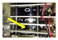
Dial up the frequency setting switch so that the 3 is just visible at the back and with some long tweezers stick on the number two in the space just above the three. (You may need a dentists mirror to see what you are doing) Ensure it is stuck well down!
