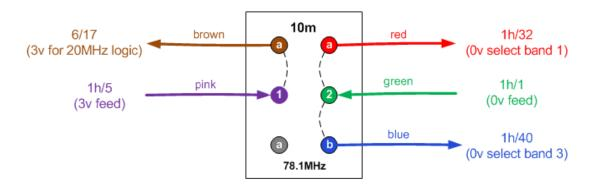
Feed the wires from the toggle switch through the looms and connect them as follows:
