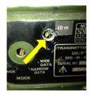
Drill a hole in the location shown just wide enough for the modification toggle switch to squeeze through (be very careful not to damage any wires when drilling and to remove any burrs and swarf from the hole once done)
