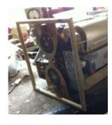
If available, fit the frame from the 353 test kit to the rear of the radio. This protects the delicate circuit boards and shaft at the end of the radio. If a frame isn't available take great care when turning the radio around on the workbench.
