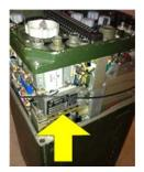
Carefully slide off the case in a smooth upward motion. It is tight fitting and if care is not taken, wires can be snagged or caught. The rubber seal may come off, don't worry too much about that, it will be replaced later.
