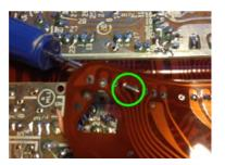
Poke the pink wire through the hole and solder it to pin 15, ensuring minimal thickness, so that a thin heat shrink can be put over it as shown below.
