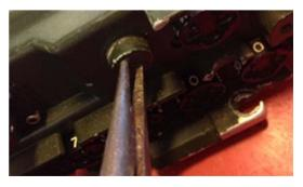
Remove (and dispose of) the drying and sealing plug as shown on the left, with a pair of snipe nosed pliers. You will probably need to drill through the hole for the toggle switch to fit through (I use a 6.5mm drill bit) As you drill, you may find the whole thread comes out or disintegrates, or stays in place.. As long as your toggle switch fits through with enough thread to screw the retaining nut on, that is fine.
