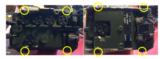
Remove the remote panel by unplugging it from the main body as shown in the picture on the right, then removing the case as shown below.
