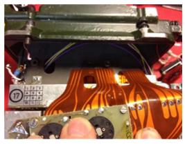
first. Gently wiggle it around until the board locates with the 25kHz switch and can be clicked through. Then do the same to the next three switches in turn until they are all in place and the screws can be replaced. Re-solder the white and black wires and put the red power plug back in position. Now screw one or two bolts in the module board to keep it in place.
